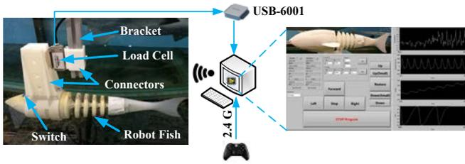
Fig. 6 The setup for the stationary experiment
